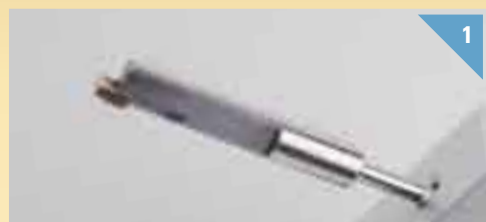
Art matrix mounted in its mandrel
