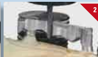
2 Finishing of the bar with a milling machine
