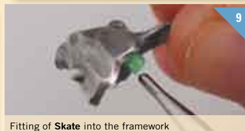
Fitting of Skate into the framework
